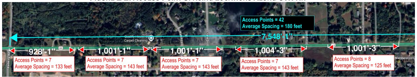
FIGURE 1-2: ACCESS POINT SPACING LOCATIONS ALONG CTH NN
