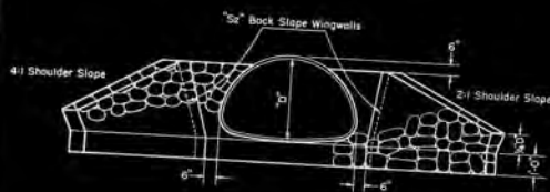
END ELEVATION SHOWING CORRUGATED METAL PIPE ARCH
