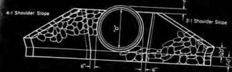
END ELEVATION SHOWING CONCRETE CIRCULAR PIPE INCL. CATTLE PASS
