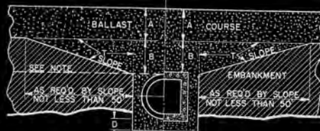
HALF SECTION - PIPE CULVERTS HALF SECTION - BOX CULVERTS TREATMENT WHEN A+B IS FROM 0 TO 5 FT. SLOPE NOT STEEPER THAN 25:1
